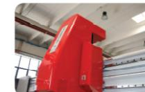
Scorrimento carrello porta disco (asse X) su guide lineari a riciclo di sfere in bagno d'olio / Disc carriage Sliding (X axis) on recirculating ball linear guides in oil bath
